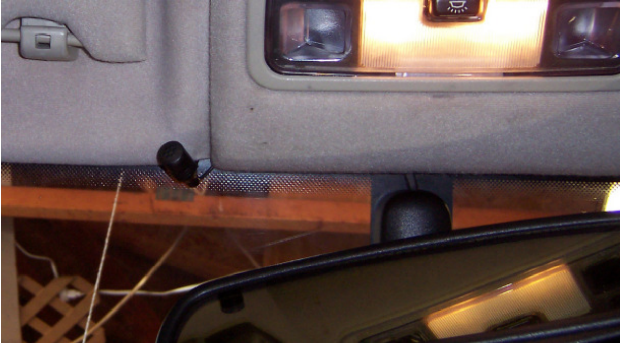
The Motorola control pad needs to be mounted in a place that the driver can easily access it. It can double back tape on it so you can stick it to any smooth surface. I chose to attach it to the drivers side of the trim around the center A/C registers.
