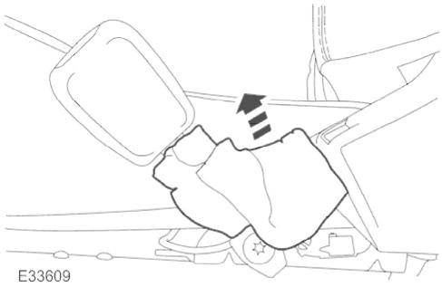
2. Reposition the seat belt buckle gaiter.
