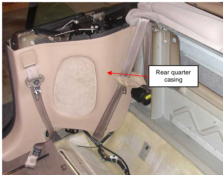
Fig. 7 Rear seat area with squab removed
