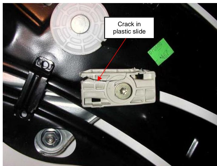
Fig. 21 Failed plastic slide
