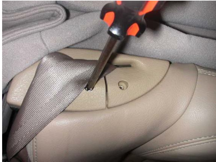
Fig. 6 Seat belt guide on seat back
