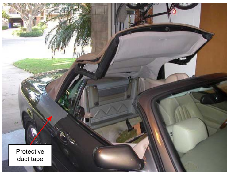
Fig. 17 Roof partially closed to allow access to top bracket cover and mounting bolts
