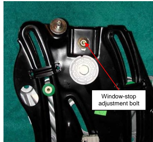
Figs. 22a and 22b View of window stop and adjustment bolt
