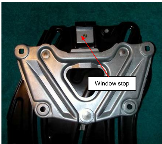
Figs. 22a and 22b View of window stop and adjustment bolt
