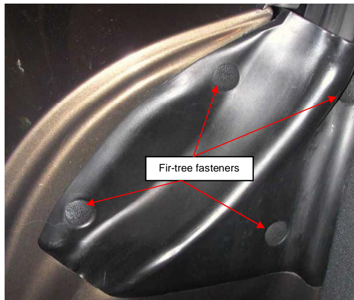
Fig. 13 Fir tree fasteners at front of window inner seal
