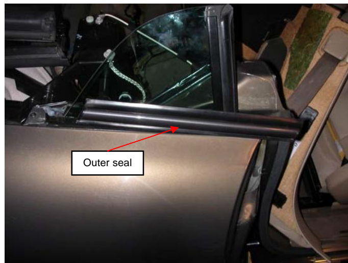
Fig. 15 Window outer seal
