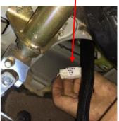
8) Check the wiring harness is free from sharp edges and moving parts. Exercise the brake light switch cam plastic trigger before releasing pedal
