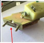
14) Zip tie harness to housing, mark back plate direction for orientation.
