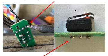
The 2 x Cherry original micros have both NO and NC contacts on each switch, however one switch is used on the (NC) side ONLY (cruise control function) and the second switch is used on the (NO) side ONLY (brake light function). The wiring harness will be soldered onto the two new switches which will be paired one on top of the other in situ after the connections are made. Throw the PCB and switches in the bin.
