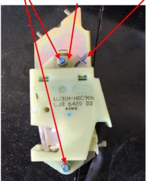
2) Mark the rotating cam position where the micros make first contact.
