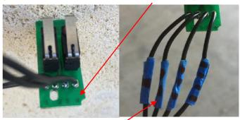
4) Marking these wires from 1 to 4 will make next phase easier.
