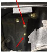
7) Locate the male and female harness plugs and apply enough pressure until they click back into position. It only fits together one way.
