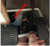
2) Cut a 180mm (7") piece of softwood to hold the brake pedal in the depressed position to allow more access whilst working below.
