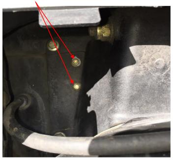
Return to the inside of the vehicle, depress the brake pedal and pull down on the brake pedal switch to remove it from the vehicle. This may take a little patience and a wiggle or two to get it out.
