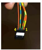
Take care to get this correct the first time. These pins are difficult to extract from the 4-position connector body. If an error is made here, please contact whitexkr@comcast.net for further directions.
