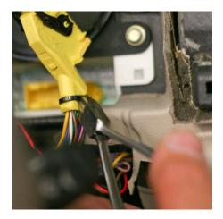
12. Pry off the hood retainer gently with a pair of pliers.
