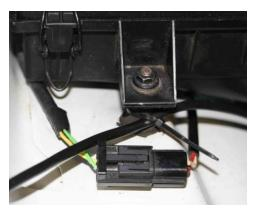
34. Remove the cover of the ECM compartment by lifting from the hole on top and pulling it away from the fender. Continue routing the sensor cable under the fender lip and into the ECM compartment. lifting the rubber block to gain access to the ECM compartment. Wrap three turns of electrical tape around the cable before inserting it in the grooves at the entrance and exit of the ECM compartment. Replace the ECM compartment cover.
