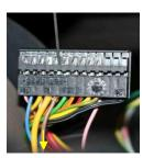
15. Check that the locking tab on each terminal stands out about 10 degrees, and bend it back into position if necessary.
