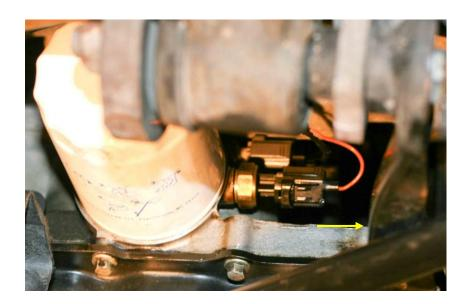
25. Remove the oil pressure switch using a 13/16" or 21mm deep socket. Have a basin or jar ready to catch the drips. Expect about 2 to 4 oz. of engine oil to drip out. Clean the mating surface on the engine block. Protective rubber gloves are recommended for this step.
