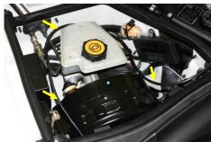
37. Pry loose the accordion rubber boot near the fender on the bottom of the brake booster compartment (see photo below). Use a flat blade screwdriver if necessary to assist. There may be a rubbery adhesive bond between the rubber and metal that you need to break. (It is not absolutely necessary, but if you have difficulty with this step remove the wipers and the plastic grille under the wipers and to gain easier access.)
