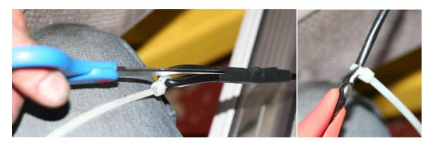
42. Route the sensor cable over kick panel mounting rail below the dashboard. Then route sensor cable up and alongside the left of the main instrument cluster and over the top of the cluster. Plug the sensor cable into the 3-pin connector on the front edge of the RealGauge module with the red wire on the left and the black wire on the right.
