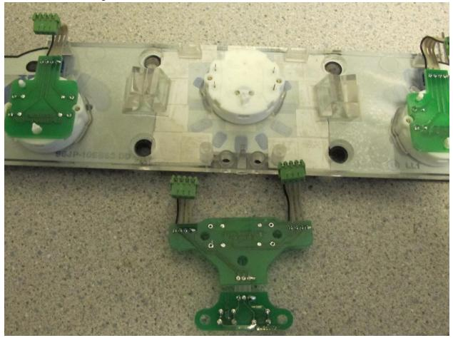
Using a solder wick or vacuum solder puller, remove the solder holding the four motor pins to the upper clock-motor board. Remove the two screws (T7) holding the extension board to the main PC board. The main PC board can now be put on one side.
