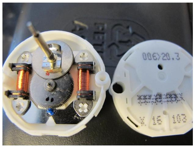
The armature / driver gear part sits on a very thin hair-like pin, fixed at the base but engaging with a tiny hole in the top cover. Using tweezers, carefully remove and discard the faulty armature / gear, similarly dismantle the purchased X-27, remove its armature / driver gear, and place it in the X-16. The two coils of the X-16 motor checked out at approximately 280 ohms each. The remainder of the X-27 can now be discarded.
