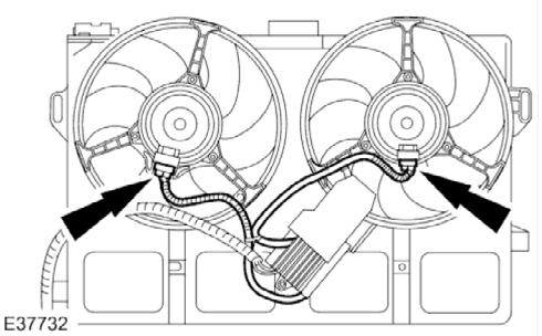
3. Disconnect the cooling fan module electrical connectors.
