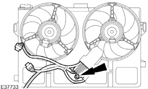
4. Remove the cooling fan module.• Remove the retaining bolt.
