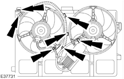
2. Detach the cooling fan module wiring harness.
