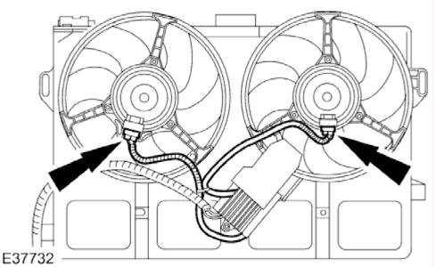
2. Connect the cooling fan module electrical connectors.
