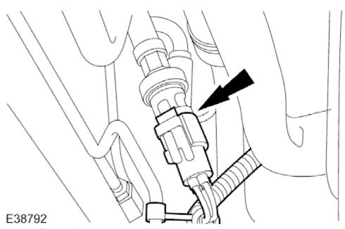
2. Connect the pressure cutoff switch electrical connector.
