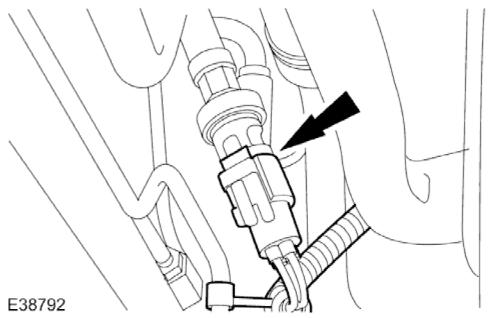
2. Disconnect the pressure cutoff switch electrical connector.
