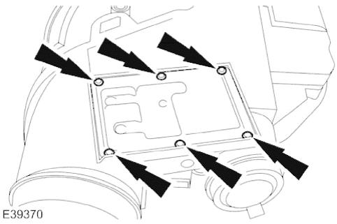
2. Remove the ballast retaining screws.
