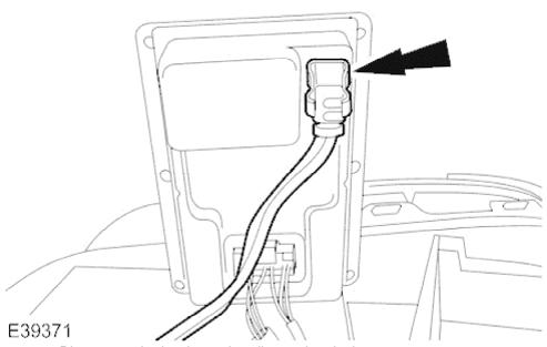
3. Disconnect the low beam headlamp electrical connector.
