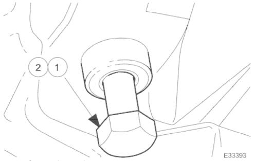
5. Separate bumper from supports.1. Slacken and remove bolts securing beam to support brackets (menasco struts on N. American market vehicles).
