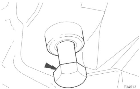
3. Fit and hand tighten beam securing bolts.
