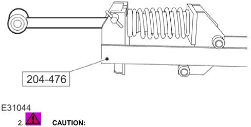
Make sure circlip on the shock absorber abuts with the lower spring pan.
