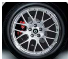
20" Perseus alloy wheels with front 255/35 ZR 20 and rear 285/30 ZR 20 Pirelli tires Standard on the XKR Victory Limited Edition
