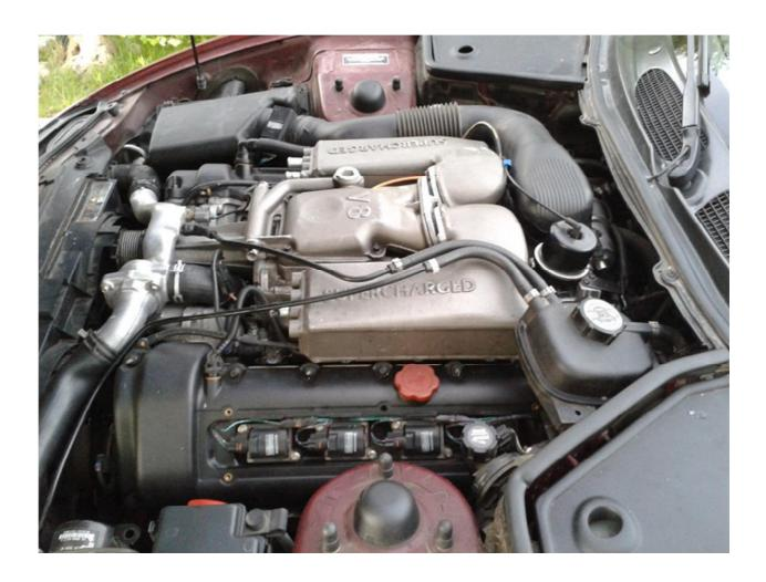
You can see that I still had the old header tank and some coolant pipes were not the perfect fit, but it was OK for the first testing.
