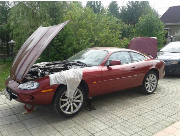
Time for the test drive! Massive low end torque is quite impressing, I've achieved right what I wanted. I've measured the AFR and despite my "high tech" MAF solution the AFR looks about right, 14.6 at idle/cruising and 10.5 at heavy acceleration. My next steps will be:
