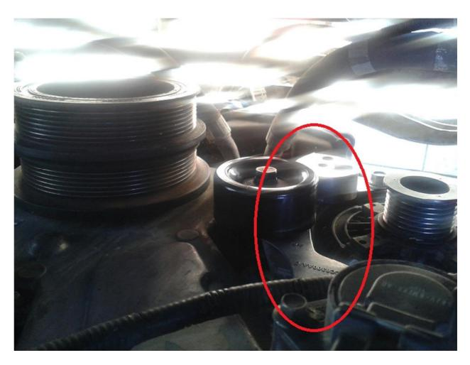
As soon as all the pulleys are in place we can install the drivebelts.
