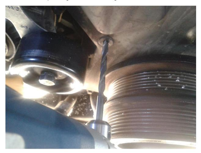
The bolts to be used are M6. It's also necessary to use some sealant around the bolts to prevent oil leaks.
